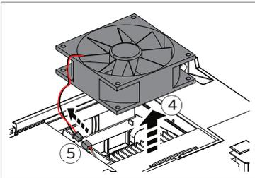
6. Replace the fan. Make sure that the air flow is in the correct direction. The air flows in from the bottom of the drive and out from the top of the drive.
