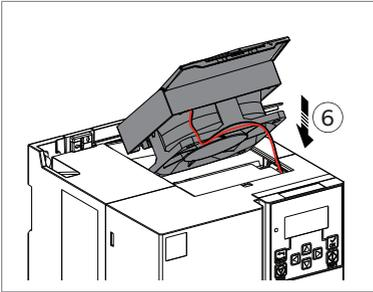
7. Carefully put the fan cover into position in the drive. Make sure that the fan power cable is routed correctly.
