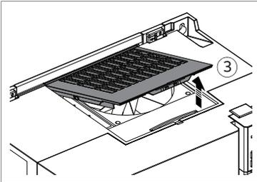
4. Lift and pull the fan from its base.
