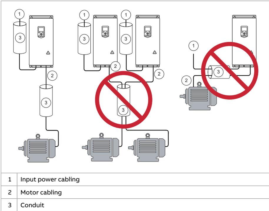
■ **Continuous motor cable shield/conduit or enclosure for equipment on the motor cable**
