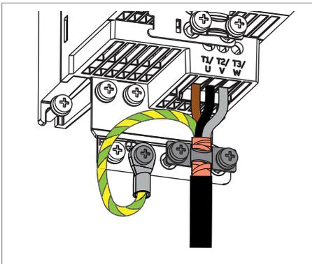
5. Twist the motor cable shield into a bundle, mark it with yellow-green and connect it to the grounding terminal.
