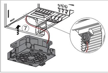
8. Carefully put the fan cover into position in the drive. Make sure that the fan power cable is routed correctly. Push the cover to lock into position.
