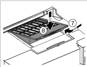
■ **To replace the cooling fan for frame size R4**
