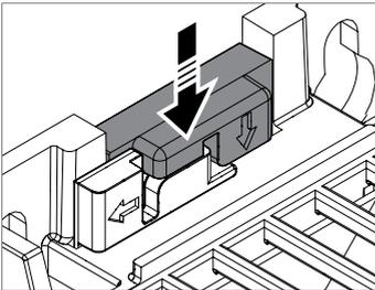
3. Put the top tabs of the drive onto the top edge of the DIN installation rail.
