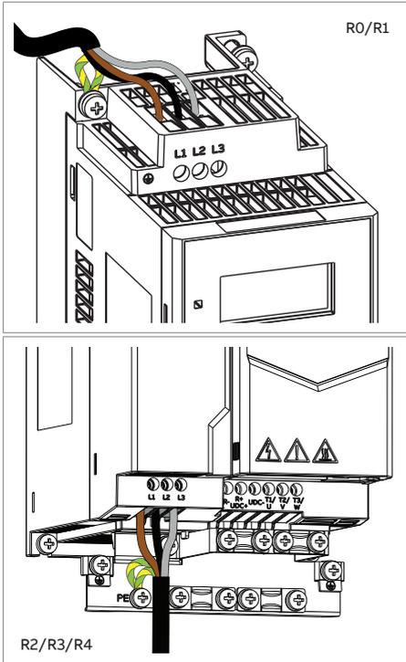
10. Mark the second grounding connector of the input side with the yellow-green and connect it to the PE terminal. (Second PE conductor is required by the drive safety standards IEC61800-5 and UL 61800-5.)
