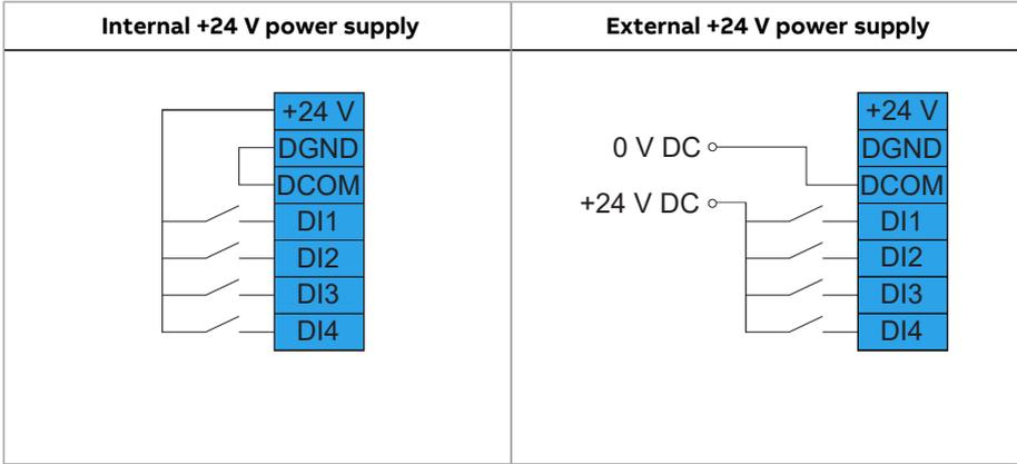
■ **NPN configuration for digital inputs**
