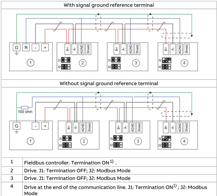
1) **Note:** The device at both ends on the fieldbus must have termination set to ON.
