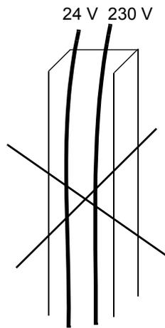
Not allowed unless the 24 V cable is insulated for 230 V or insulated with an insulation sleeving for 230 V.
