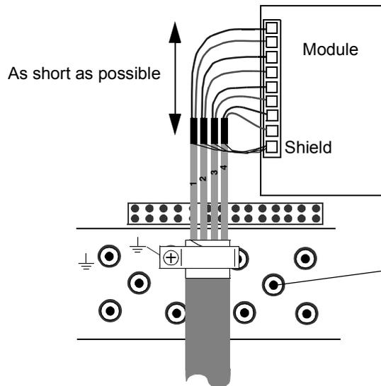
**Note:** The RDIO module does not include a terminal for cable shield grounding. Ground the pair cable shields here.
