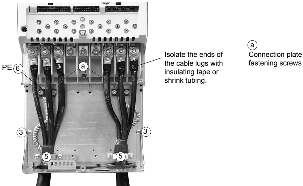
Frame size R6: Cable terminal installation [95 to 185 mm<sup>2</sup> (3/0 to 350 AWG) cables]
