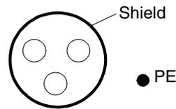
A four-conductor system: three phase conductors and a protective conductor.
