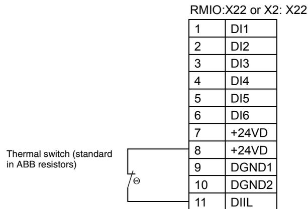
For other application programs, the thermal switch may be wired to a different digital input. Programming of the input to trip the drive by “EXTERNAL FAULT” may be needed. See the appropriate firmware manual.
