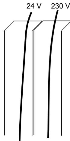
Lead 24 V and 230 V control cables in separate ducts inside the cabinet.
