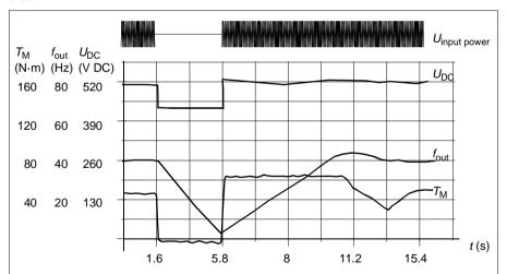
$U_{DC}$  = Intermediate circuit voltage of the drive,  $f_{out}$  = Output frequency of the drive,  $T_{\rm M}$  = Motor torque
